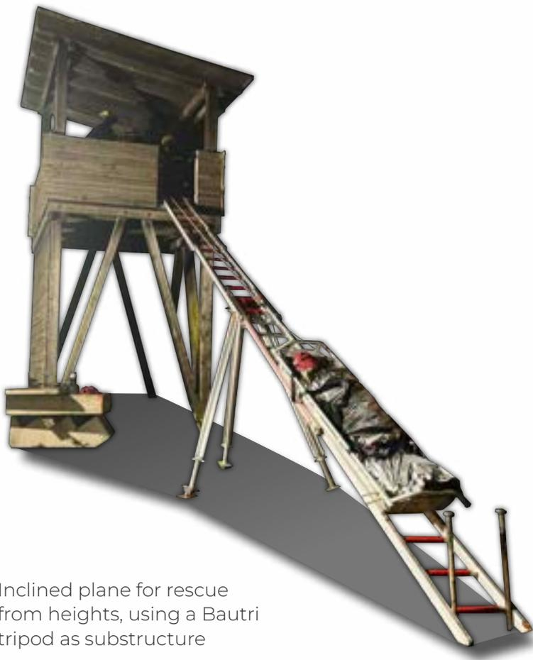
Inclined plane for rescue from heights, using a Bautri tripod as substructure
