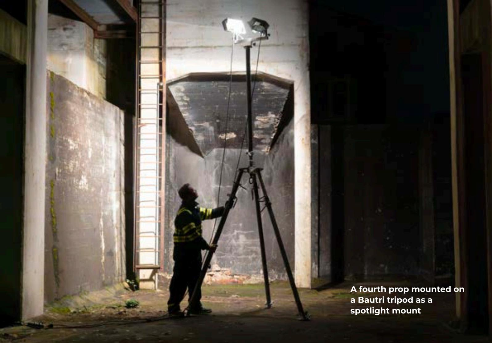
A fourth prop mounted on a Bautri tripod as a spotlight mount
