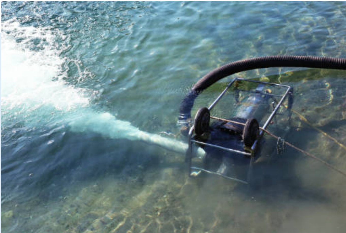
VenturiPulse in use on a Wilo-Drain TP 100E submersible pump
